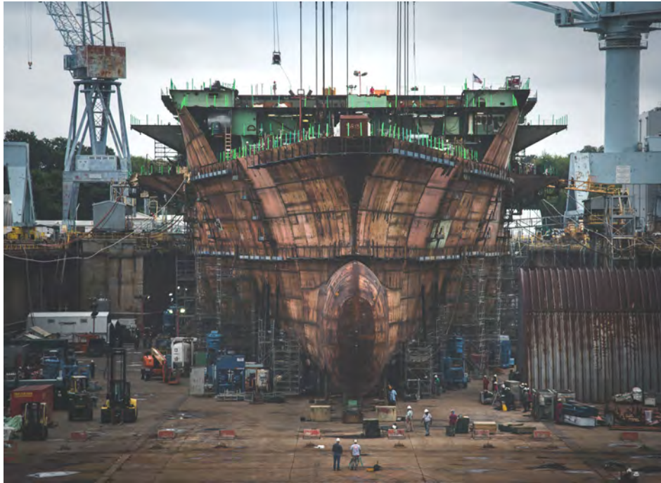
CVN 79 Underwater Hull in Dry Dock. Courtesy of Huntington Ingalls Industries - Newport News Shipbuilding.
