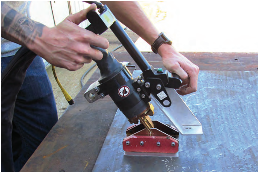
Induction heating and straightening for ship panels will reduce rework. Courtesy of NSAM
