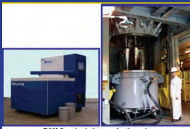
RAM-5 and existing production mixer
