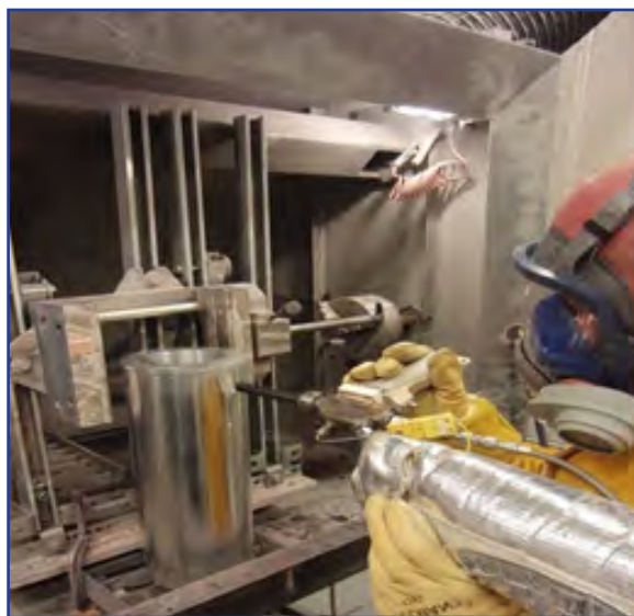
Innovative Cold Spray Repair Technology for Ships. Courtesy of iMAST
