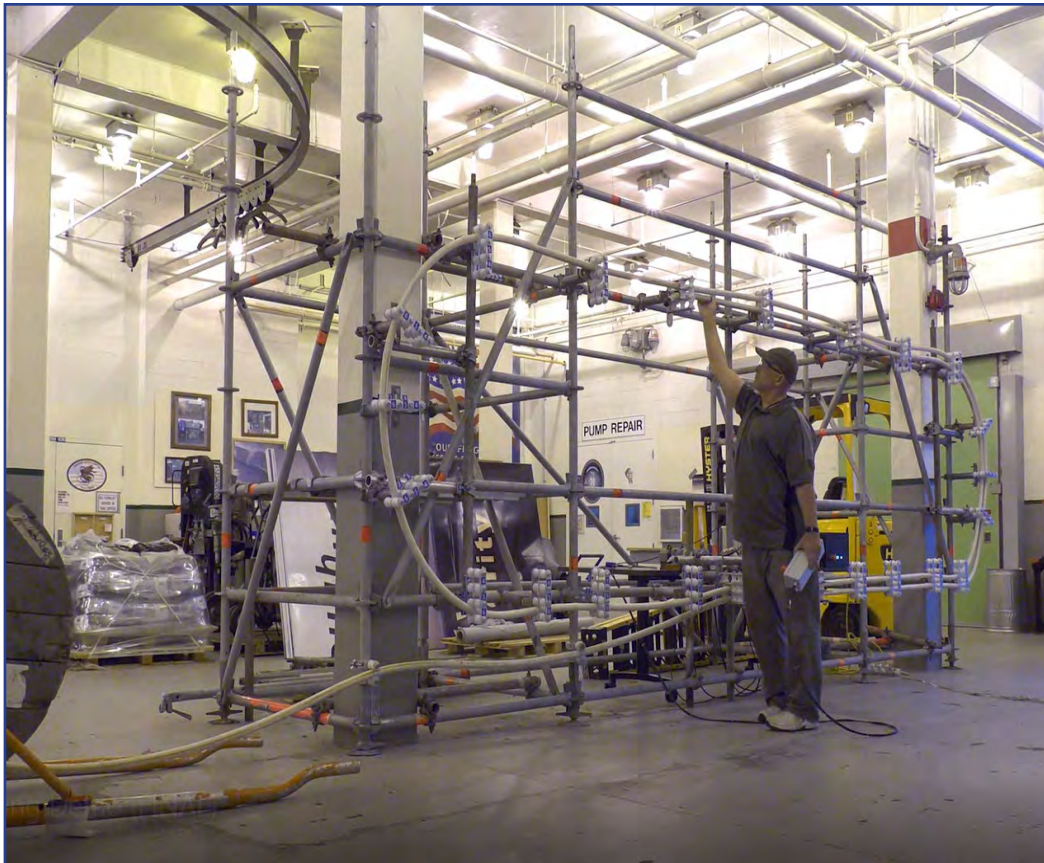
Synchronized Cable Feeding System Expected to Reduce Cable Installation Cost. Courtesy of iMAST
