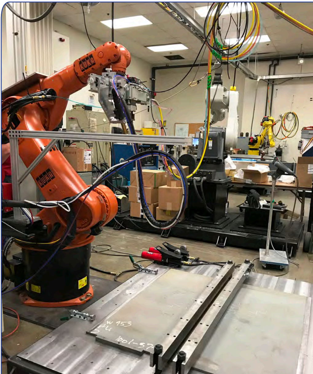
Hybrid Laser Arc Welding – Courtesy of Huntington Ingalls Industries - Ingalls Shipbuilding / NSAM
